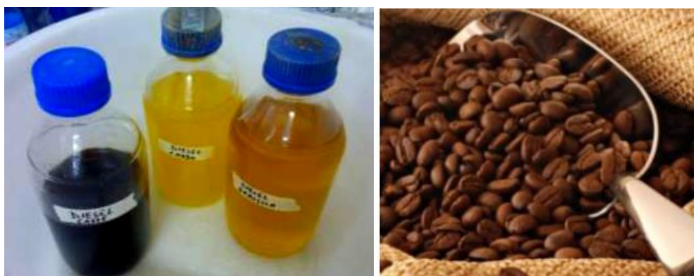
Figure 1. Coffee beans on the right and used biodiesel fuels derived from the Cynara cardunculus (orange colour), Brassica carinata (yellow colour) and Coffee (black colour) in the bottles on the left.
