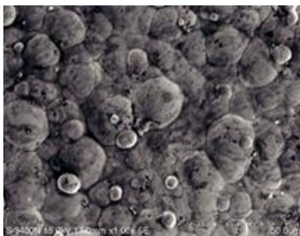
Figure 5. EN-P bath A without Nano additives.
