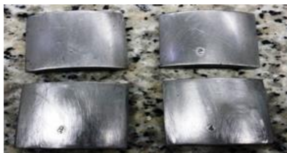
Figure 2. Samples after mechanical & chemical polishing.
